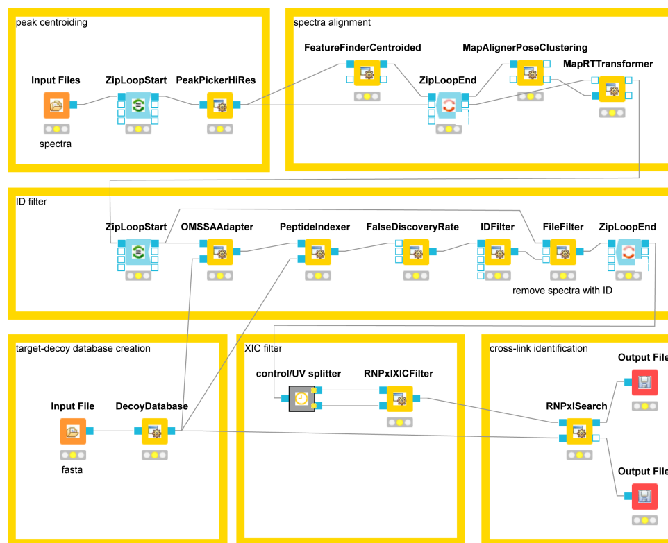
Figure 3.19: OpenMS workflow for cross-link identification and localization using the RNP x1 Search engine in KNIME. The workflow consists of target-decoy database creation, peak centroiding and chromatographic alignment, ID/XIC filter, and cross-link identification. Orange nodes indicate input files(s), yellow nodes TOPP tools, red nodes output files(s). Nodes are connected by edges that indicate the flow of data. Between corresponding ZipLoopStart/ZipLoopEnd nodes, a list of files is sequentially processed.
