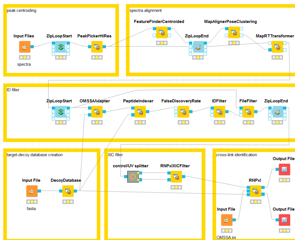
Figure C.4: OpenMS workflow for cross-Link identification using the RNP xl tool in KNIME. Workflow consists of target-decoy database creation, peak centroiding, chromatographic alignment, ID/XIC filter and cross-link identification. Orange nodes indicate input files(s), yellow nodes TOPP tools, red nodes output files(s). Nodes are connected by edges that indicate the flow of data. Between corresponding ZipLoopStart/ZipLoopEnd nodes, a list of files is sequentially processed.
