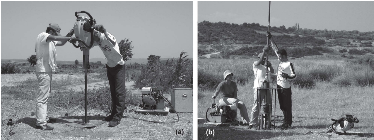
Fig. 12 A gouge-corer drilling operation. Percussion drilling gun (a), Cobra, provides driving 1 m gouge corer into ground. To go deeper, 1 m extension rods are attached each time. Then hydraulic lifter (b) provides to pull up rods and corer to obtain sediment core (see Fig. 13).
