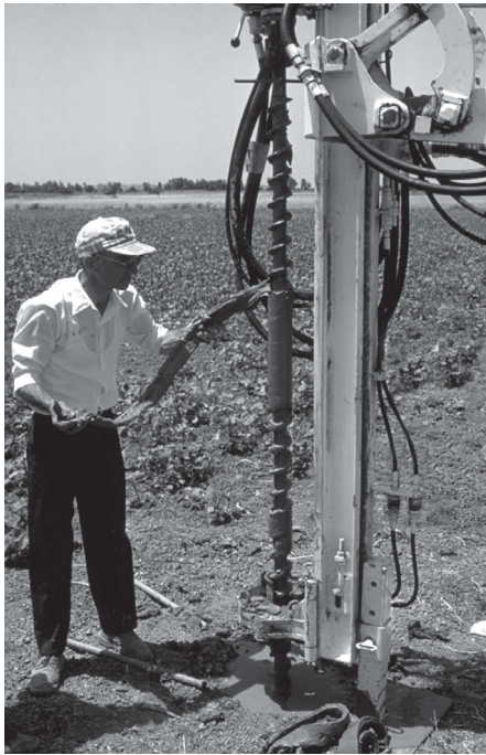
Fig. 11 Sediment examples on screw-corers taken by Unimog. These are disturbed because of compression and driven upward during the operation in the hole. Cohesive sediments can be taken from the corer as in a block shape, while loose sandy sediments unload and good sampling is not possible.
