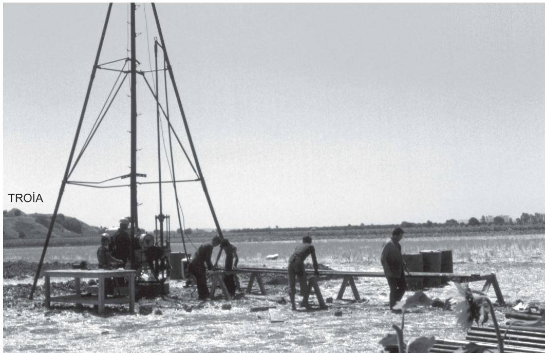
Fig. 3 An operation of a rotary core drilling (ÇKM 4) to the north of Troia. This drilling performed by MTA in 1977 obtained a good stratigraphical profile. The Miocene bedrock surface was encountered at a depth 37 m below present surface, which is about 7 m above sea level. Lower 15 m of the sediment profile indicates marine environment. Above this, about 8 m deltaic and then 7 m fluvial-terrestrial sediment units ensue each other vertically (see also Fig. 15).
