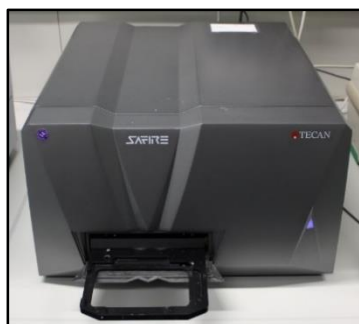
Figure 14. The Tecan Sapphire plate reader used for the absorbance measurements.
