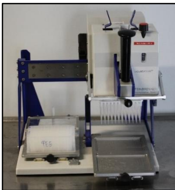
Figure 15. The Liquidator multi-pipetting system.
