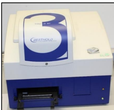
Figure 16. Berthold plate reader used for fluorescence and luminescence measurements.
