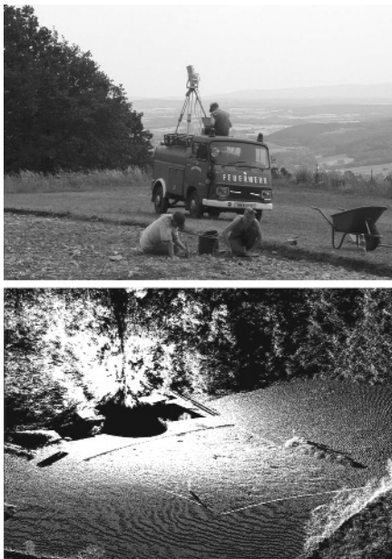
Figure 4: 3D laser scanning for the documentation of single surfaces at the excavation Schwarzenbach. Upper left: Laser scanner in action. Lower left: Intensity image of a RIEGL LMS-Z210 laser scanner showing the excavation. Upper right: comparison between data and TIN using a total station (left) and a laser scanner (right). Lower right: Visualization of the surface
