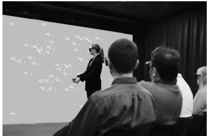
Fig. 6. Power wall. 3D stereoscopic view of underwater environment for multiple seated participants.
