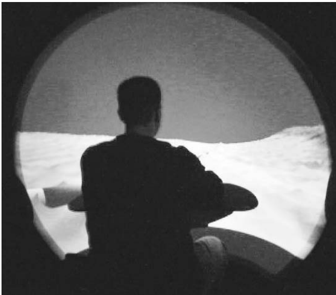
Fig. 8. User sitting in hemisphere display that can be used as an effective virtual submarine 'glass bubble' window into the marine environment.
