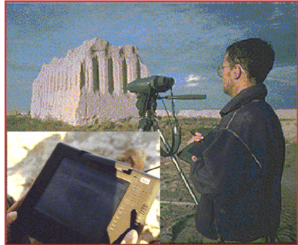
Figure 12. Leica Vector ranging binoculars with PenMap.
