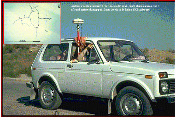
Figure 7. GPS antenna vehicle mounted with inset showing field plot of surveyed road network.
