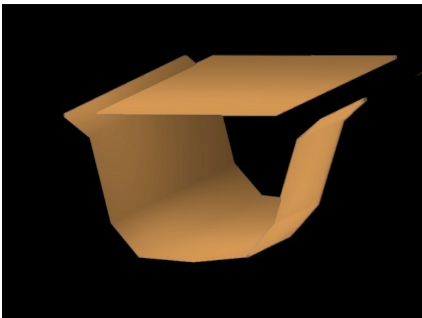
Figure 2: Surfaces which define the volume of the fill of the later trench in our model. The top surface is scanned before the fill is removed. The lower surface is scanned when fill has been excavated and demonstrates how the exact edge where the 2 surfaces should theoretically have met is lost through overcutting.
