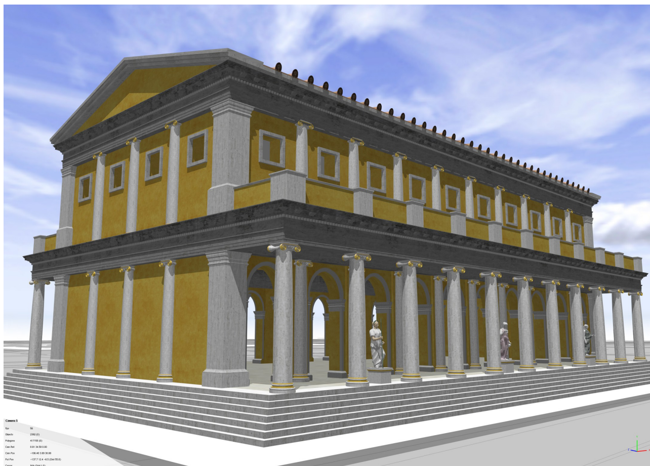
Figure 6: The roman "Basilica" in the workspace. The model was generated at high level of detail with procedural technique. Architectural details, as columns, statue, pillars and friezes, was imported form Blender software.
