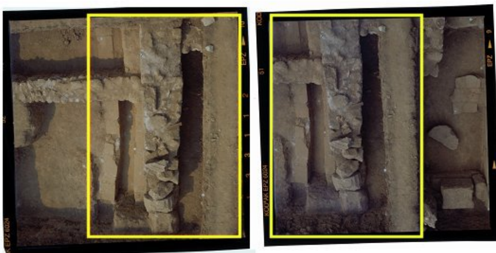
Fig. 1. Left and right images of a stereo model and their overlapping region
