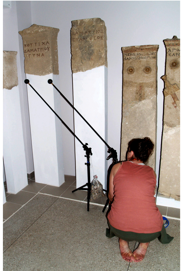
Figure 6. Positioning the reflective spheres for the capture of an RTI of a stela displayed in a tight corner (photo by Kira Zykova).
