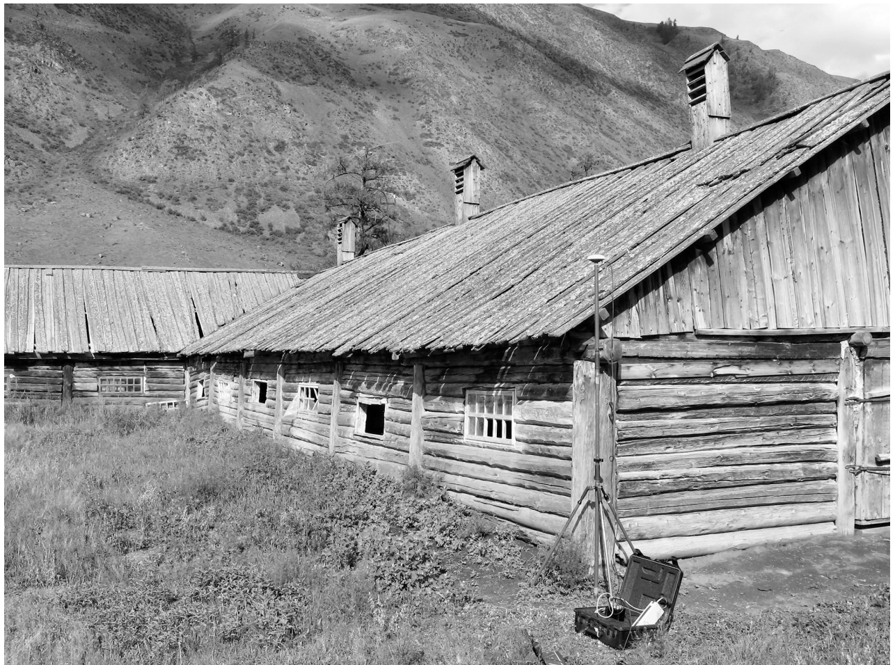
Figure 2. Measuring ground control points with the C-Nav GPS receiver.
