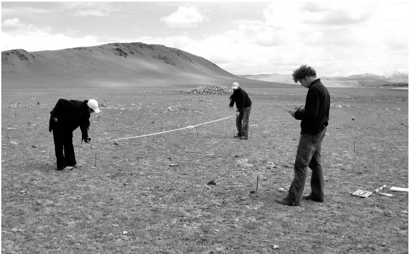
Figure 5. Measuring in the field with decimeter and goniometer.
