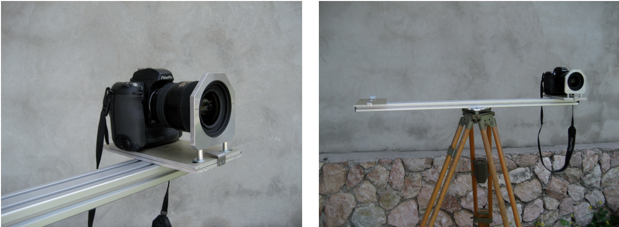
Fig. 7. Simple basis for taking stereo models.
