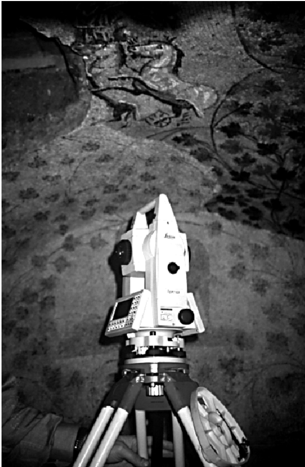
Figure 1: Total laser station for the topographic survey.
