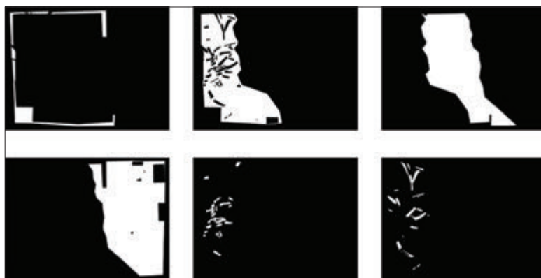
Figure 3. Examples for classification masks. The masks are used for the image-based classification and determine if the area covered by a certain pixel belongs to a semantic entity (white) or not (black).
