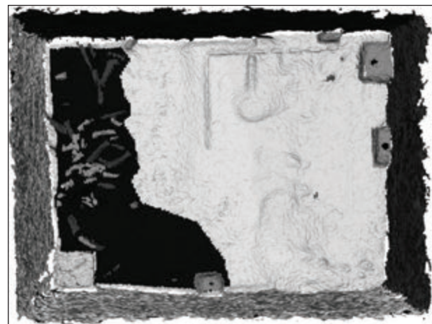
Figure 9. The resulting semantic classification. The layer is classified into the entities contained in the CAD drawing. Additionally, the profiles (which are semantic entities too) are segmented based on the surface normals.
