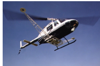
Fig. 2. FLI-MAP 400 Helicopter LiDAR system (Fugro).
