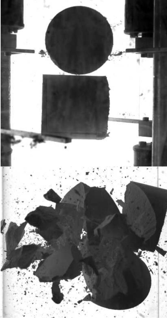
**Figure 3.** Top: the two dust agglomerates shortly after release and before the collision. Both release mechanisms are fully open. Bottom: the two dust agglomerates fragment shortly after impact.
