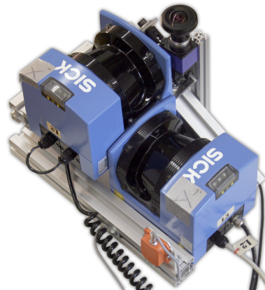
Fig. 7 Prototype system of the proposed setup consisting of two 2D laser scanners and an XSense inertia sensor. The prototype additionally includes a color camera with fisheye lens to capture texture information.
