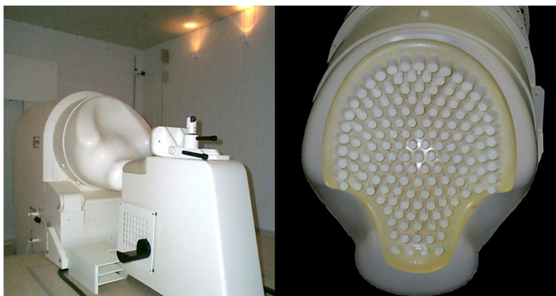
Figure 1.8: The SARA I system. Left: General view of the system. Right: the concave array of sensors. The image is courtesy of UAMS, Sara Research Center, Little Rock, USA and CTF Corporation, Canada.
