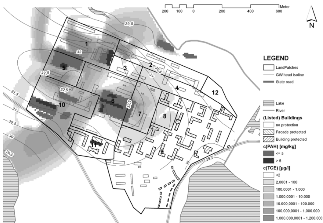
Figure 1.1: Case study site data: Information about groundwater regime and subsurface contamination, existing buildings, state roads, and water bodies, as a basis for subdivision into 12 planning units (“land patches”).
