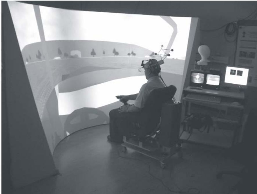
Figure 1. Image of the experimental set-up. Study participant performing collision avoidance in front of the projection screen.
