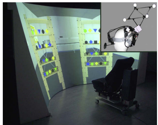
Fig. 1. Image of the curved projection screen and the displayed comparative visual search paradigm (cupboard task). Subjects sit comfortably in a high adjustable seat while performing the experiments. Small picture: ASL501 eye tracker with fixed rigid body enabling head tracking.
