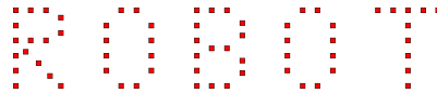
Figure 6.1: Five desired formation configurations: R O B O T. Squares represent the target positions in the formation. The number of positions M are equal to 16, 12, 16, 12, and 10, respectively.
