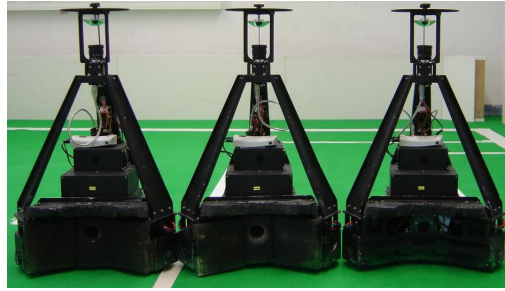
Figure 5.4: Omnidirectional mobile robots used in the formation control experiments.
