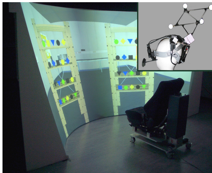
Figure 1. Image of the curved projection screen and the displayed comparative visual search paradigm (cupboard task). Subjects sit comfortably in a high adjustable seat while performing the experiments. Small picture: ASL501 eye tracker with fixed rigid body enabling head tracking.
