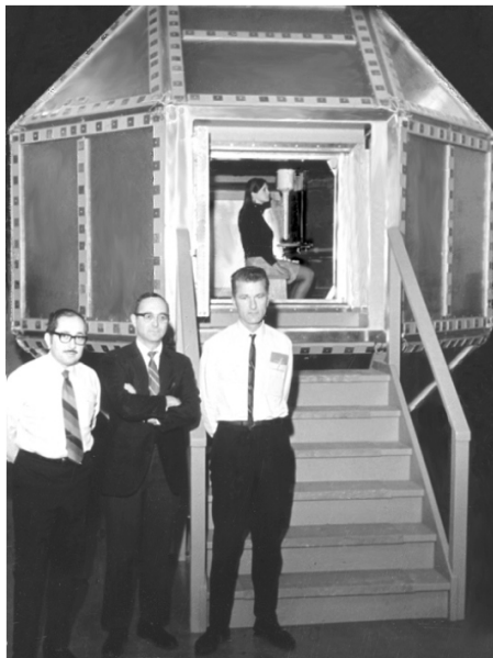
Figure 2.9: The first MEG system using a SQUID in a shielded room was operated at the Francis Bitter Magnetic Laboratory at MIT by David Cohen, Ed Zimmermann and Jim Zimmermann in 1969 (reproduced with friendly permission of D. Cohen).
