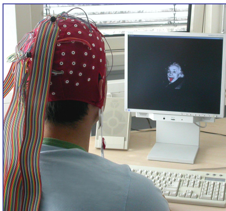
Figure 5.2: Subject with applied EEG cap that provides up to 128 electrodes. The screen displays a cue for a movement imagery task (here: imagined tongue movement).
