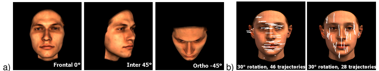
Figure 1.6: Effects of horizontal and vertical rotation on images faces. a) For a vertical rotation of 45^\circ , many distinct features of the face are severely foreshortened or even lost as opposed to a horizontal rotation of the same angle, where the features are still visible. b) Tracking of features across 30^\circ horizontal and vertical rotation.
