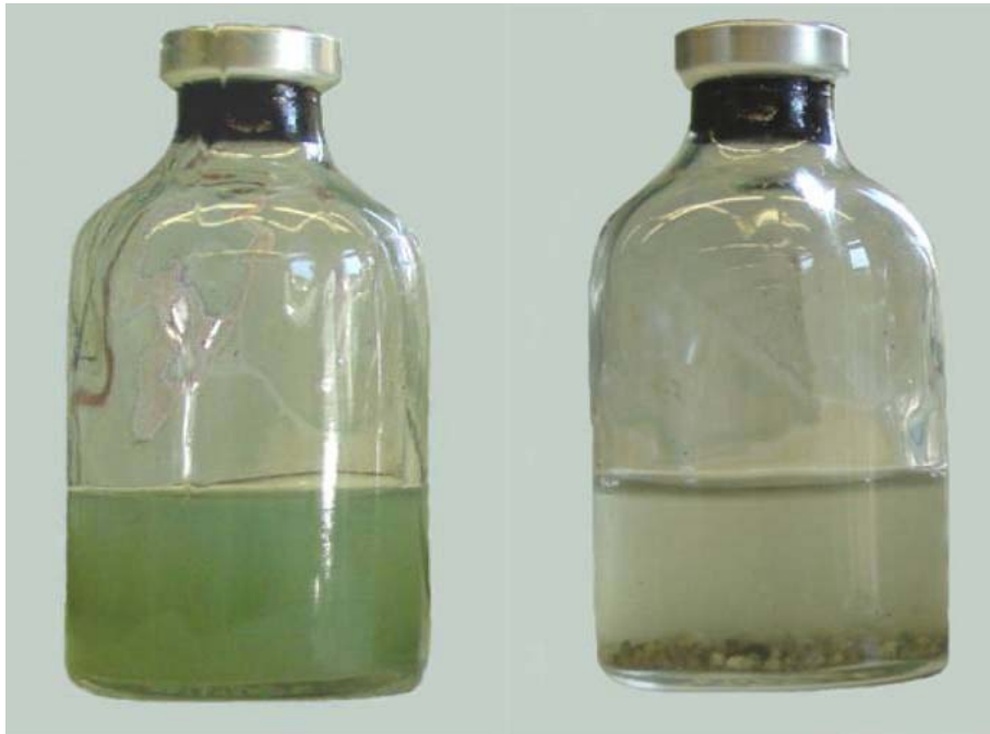
Figure 3.2 B): Reduction of Prussian Blue in a natural sandy soil sample by Geobacter metallireducens cells. The culture contained sodium acetate as sole carbon and electron source and Prussian Blue coated sand as sole electron acceptor. The bottle on the left shows the culture after shaking the sand sample over night in the culture medium before incubation. The blue colour of the colloidal Prussian Blue particles in the supernatant is clearly visible. The bottle on the right shows the same culture after several hours of incubation with the bacterial cells. The blue colour has completely disappeared.
