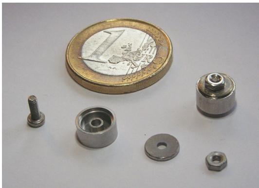
**Fig. 5-2:** Photograph of stainless steel capsules (dismantled and closed) used during this study to load apatite crystals.
