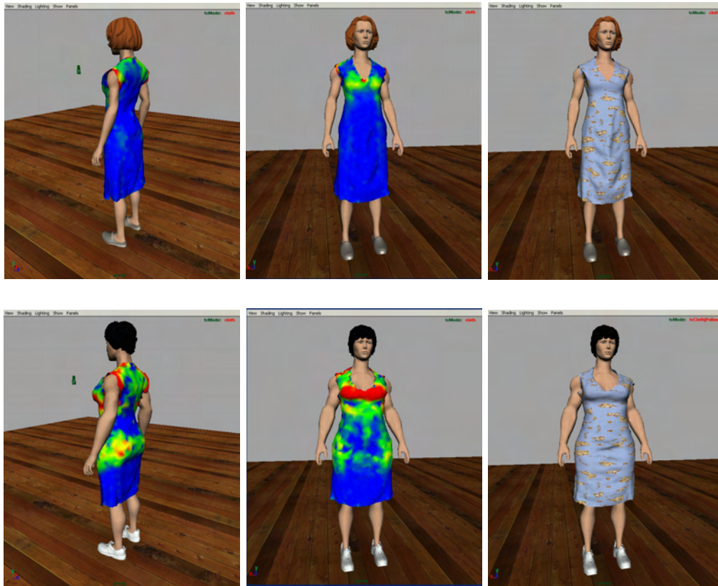
Figure 6.4: A dress tried-on by two women with different body proportions. The internal forces are visualized with colors from red to blue representing high to low tension forces. For the woman in the upper row, low tension forces result, i.e. the dress fits well. It is however too small for the woman in the lower row.
