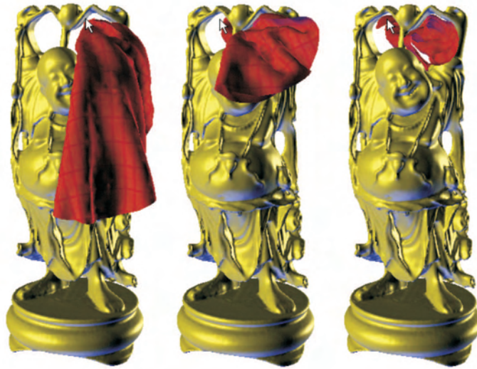
Figure 2.6: Interactive animation of cloth using the distance field of the Happy Buddha (Figure 2.4 for collision detection). Image courtesy of A. Fuhrmann, IGD Darmstadt.
