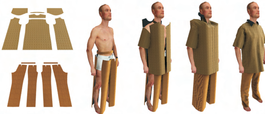
Figure 6.2: The pre-positioning and simulation steps of the pipeline realized in the bmb+f project Virtual Try-On.
