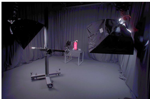
Figure 8.2: A view of our photo studio with black, diffuse reflecting material on the floor, walls, and ceiling. This image was generated from a High Dynamic Range image to which a tone-mapper has been applied.
