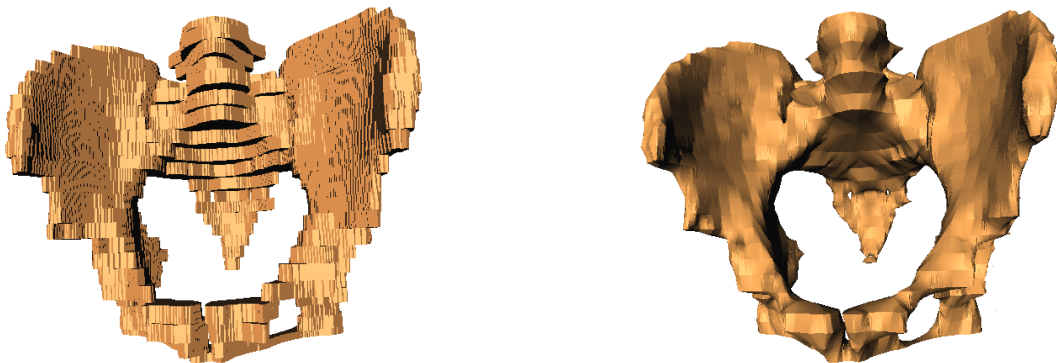
Figure 2: Reconstruction of a hip from 23 contours. The dataset is publicly available from Tel Aviv University. On the left side the contours are simply filled ( 300 \times 300 grid). On the right side a distance field was calculated using the new algorithm. Both surfaces were extracted with a standard MC-algorithm. The times for generating the distance-fields are reported in 1.
