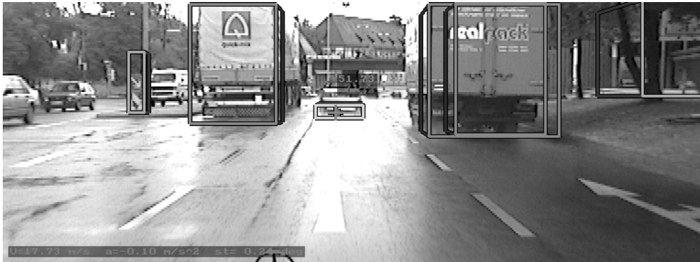
Figure 7.17: Traffic scene with trucks to the left and right of the leader vehicle. Back light, wet street, and a large distance deteriorate detection.
