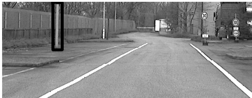
Figure 5.8: Back court scene to test the ego-position estimation algorithms. The landmark used for ego-position estimation is the lamppost with the black rectangle drawn around it.
