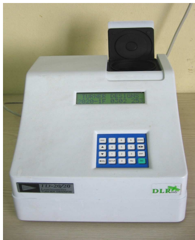
Figure 10. Luminometer for the intracellular ATP measurement by luciferin-luciferase assay (TD-20/20 Turner Designs, Sunnyvalde, CA, USA)
