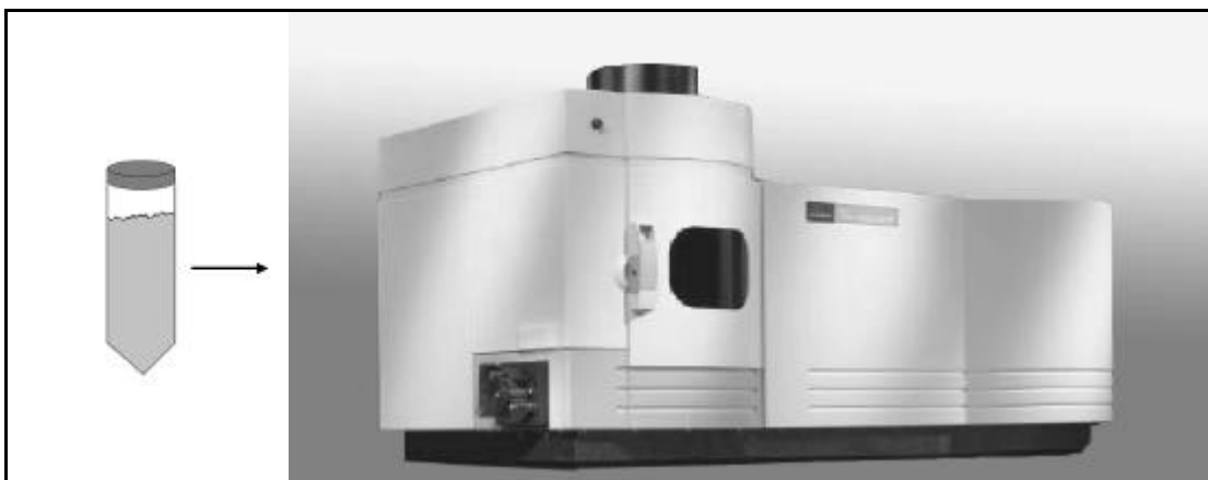
Figure 3: The conditioning media was analyzed by ICP-OES for the presence of the elements of interest.
