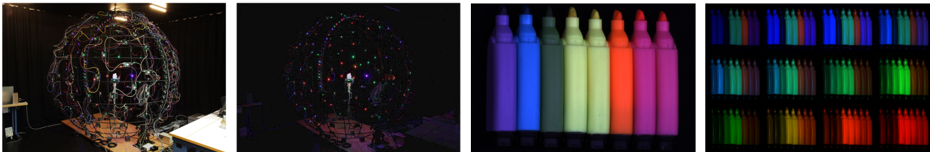
Figure 1: The LED-based hyperspectral light stage can emit a different controlled spectrum from each light source direction simultaneously enabling compressive bispectral measurements of reflectance fields. One slice showing different illumination wavelengths and directions is shown on the right for a set of text markers. The compressive sparse and low-rank reconstruction approach robustly estimates a low-rank approximation plus a sparse representation for the non-low-rank content for 14 wavelength bands and 196 directions from only 400 captured samples.
