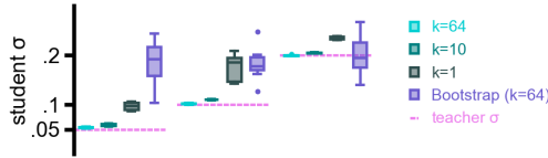
FIGURE .14: Our method allows recovering the true latent noise in student-teacher setups. We repeated the experiment of Fig. 4.3a for teacher networks with three levels of latent noise, with diagonal covariances matrices \Sigma_z = \sigma^2 \mathbf{I} . For each teacher we trained 5 student networks with varying number of particles ( k ), as well as using the bootstrap proposal (i.e., sampling from the prior). The standard deviations \sigma of the latent noise process only matches between the student and teacher, if we use enough particles during training. The bootstrap proposal (with k=64 ) is not as reliable as the optimal proposal.
