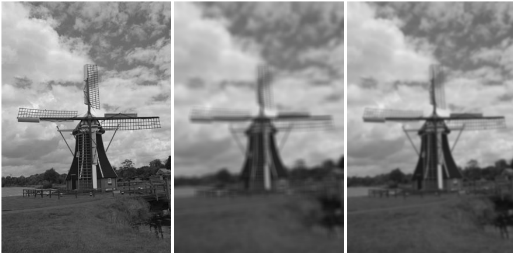
FIGURE 2.2: Examples of smoothing filters from left to right: Original image; Box filtered image; Gaussian filtered image. The mask size for both filters was 9 \times 9 .
