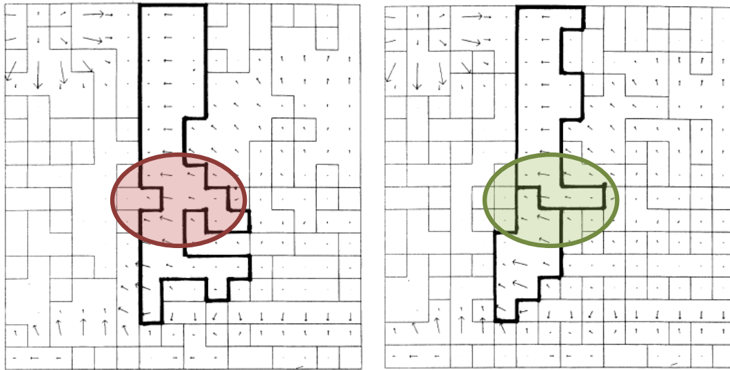
FIGURE 8.2: Example of over-merging. Left - Too large bins, region is merged. Right - Smaller bins, region is not merged.
