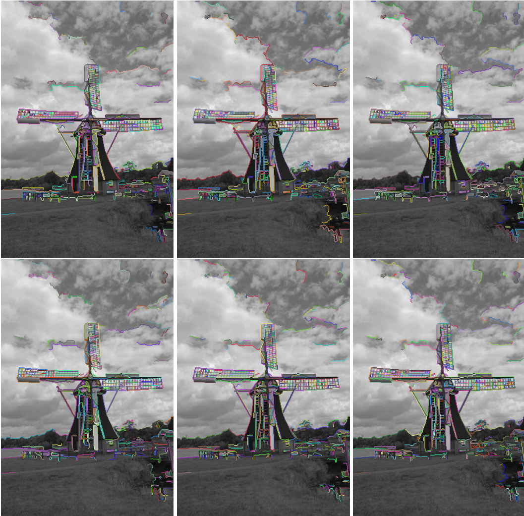
FIGURE 7.10: Examples for all edge methods. Top left to right: Edge Simple, Edge Linking and Edge Pattern Linking. Bottom left to right: Edge Drawing, Edge Linking with corner rule, Edge Pattern Linking with corner rule. The images show the results of the non-maximum suppression (NMS) step processed with Otsu estimated thresholds. The coloring is chosen at random to distinguish the segments.
