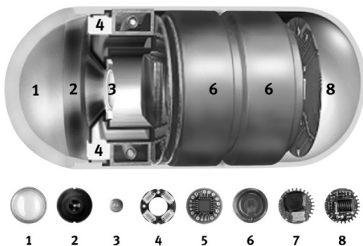
(A) M2A™ from Given Imaging Ltd. with an optical dome (1), lens holder (2), lens (3), LEDs (4), CMOS imager (5), battery (6), Application-Specific Integrated Circuit transmitter (7) and antenna (8) from [Yu02]
