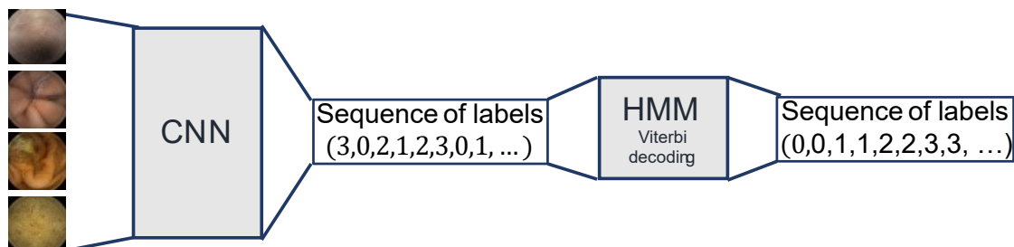
FIGURE 3.4: VCE Image processing pipeline using a CNN, a HMM and Viterbi decoding, from [Wer+23].
