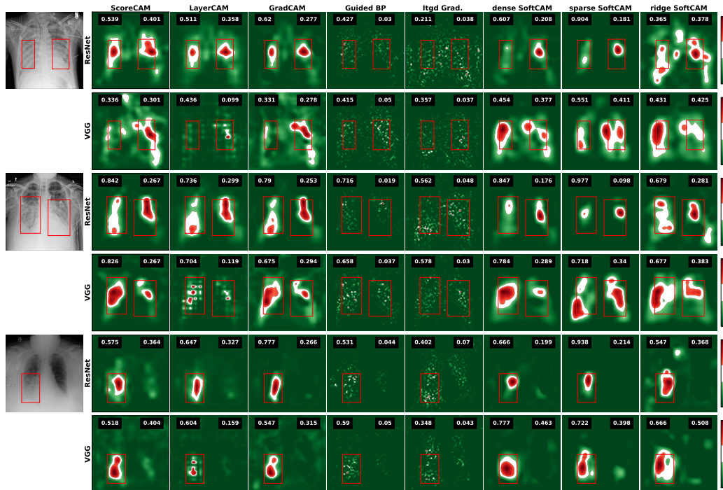
Figure 12: Additional examples of localization evaluation on the RSNA dataset for pneumonia detection. Each column shows explanation maps generated by different methods. Ground-truth bounding boxes are overlaid on each map, with the top-right value indicating the activation precision, while the top-left value indicates the activation sensitivity. The high precision from the lasso model and the more complete explanations from the ridge model emphasize the importance of balancing the two regularization terms to achieve an optimal trade-off.
