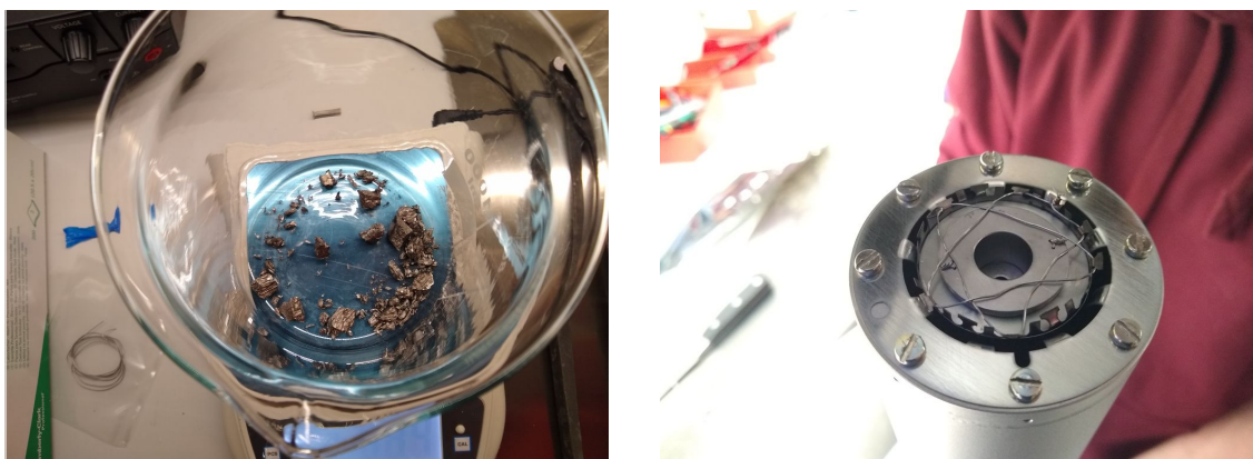
Figure C.2 | Filling and closing the Er oven. Approximately 100 g of Er chunks (left) were placed in the oven. After placing the small chunks in the crucible, it is maintained in place at the exit of the oven by a Tantalum filament (right, star shaped).
