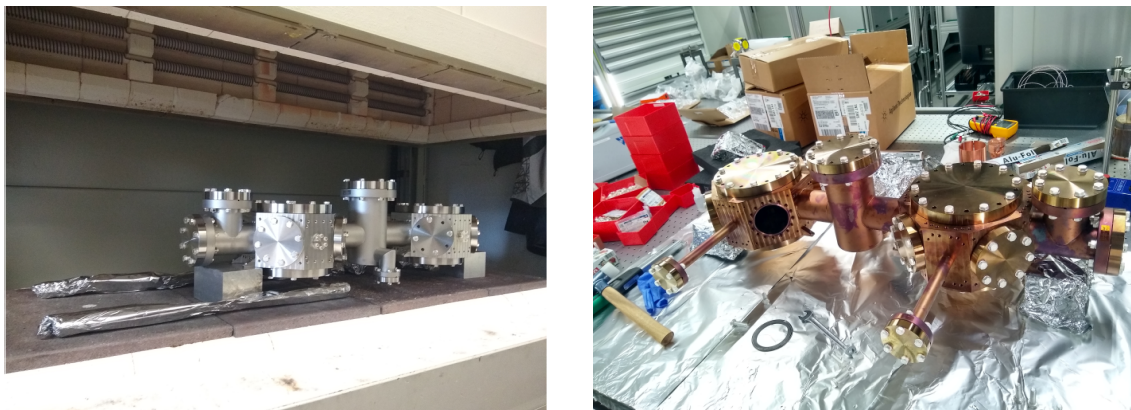
Figure C.1 | Air baking of the main vacuum chamber The main vacuum chamber was placed in a large oven (left), to be air-baked at 450 °C for 24 h. After the air-baking, the surface is oxidized and now has a bronze color (right).
