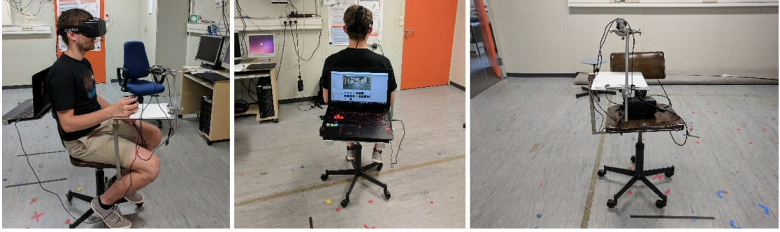
Figure 2.1: The setup for the experiments consists of a modified rotating chair. Attached to the chair is a small desk for carrying a laptop and a tablet arm desk for drawing the sketch maps. Attached to the tablet arm desk is a camera stand with camera that captures a live video from the sketch paper that is displayed in the virtual environment.
