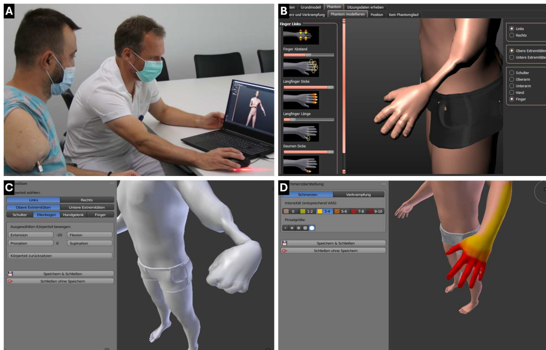
Figure 3.1: (A) A patient and a therapist are modeling the patient’s phantom limb with the CALA prototype. (B) An avatar could be adjusted, and the shape of the phantom limb could be modified. (C) A Blender plugin was used to adjust the phantom limb’s position. (D) A further plugin enabled painting pain and cramps directly on the avatar.
