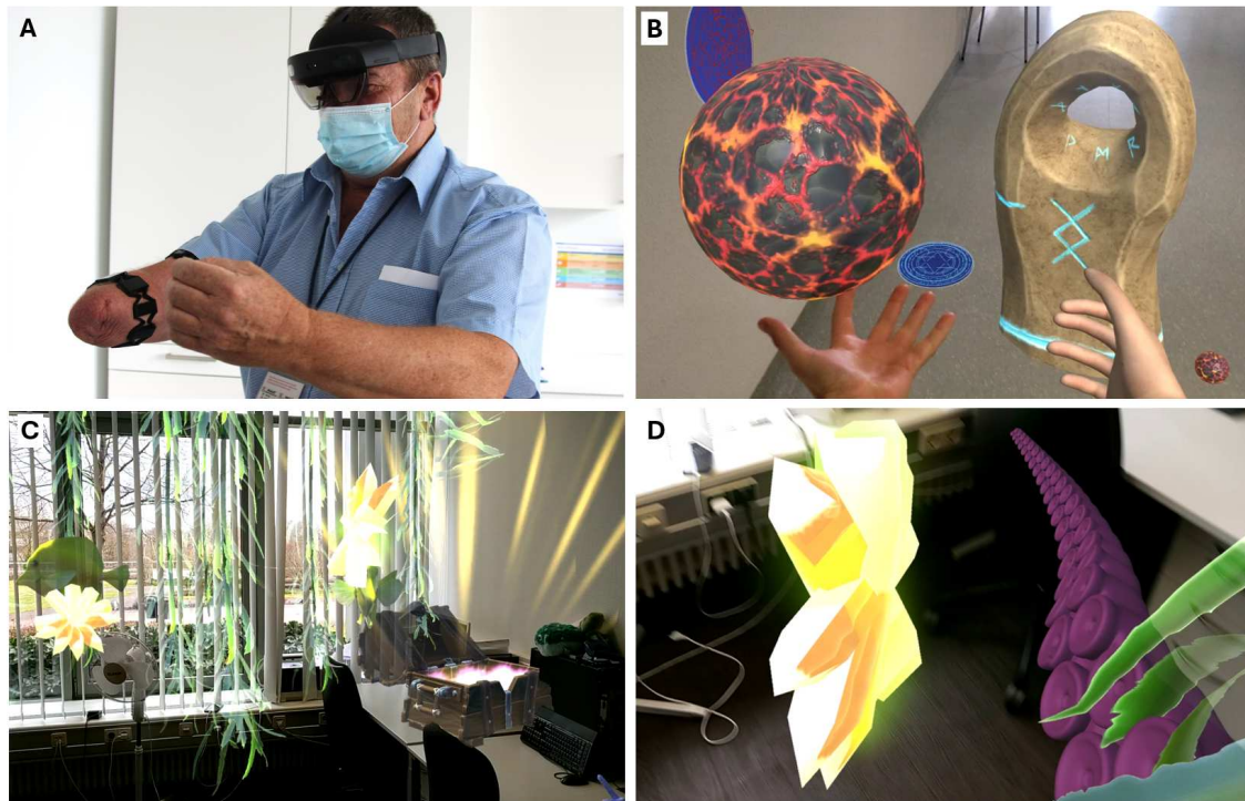
Figure 5.1: (A) A patient plays PhantomAR, equipped with a Microsoft HoloLens 2, a Thalmic Labs Myo Armband around his stump and another one around his upper arm. (B) Virtual objects could be manipulated with the real and the virtual hand (from Prahm et al. (2025), Journal of Neuroengineering and Rehabilitation , CC BY 4.0). (C) All environments were dynamically generated based on the real surroundings, using walls, the floor and desks. (D) A tentacle was used to evaluate the effects of using a non-anthropomorphic representation of the phantom limb in comparison to a human hand.
