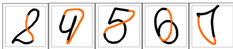
Figure 6.5.: Examples of training sequences for symbol classes "2", "4", "5", "6", and "7". Augmenting data (orange pixels) were appended to the original curves (black pixels) to form closed-loop curves with a smooth transition between the original and augmented segments.
