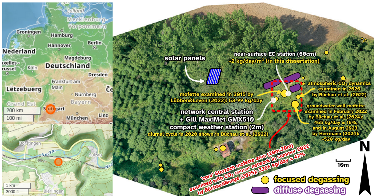
Figure 1: Overview of the Starzach site in southwestern Germany, highlighting the spatial distribution of its CO 2 degassing activity, the deployed measurement equipment, and relevant emission quantification studies with estimated CO 2 emission rates given in kg d -1 . Figure adapted from Büchau et al. (2022, Appendix A, page 61, kindly provided by the publisher under a CC-BY-4.0 license), with the following changes: Annotations of the aerial imagery on the right-hand side (drone photogrammetry from 2019 by Martin Schön) were updated, and the maps on the left-hand side were replaced with current views from OpenStreetMap.org ('Tracestrack Topo' layer, 16.10.2025). Map data © OpenStreetMap contributors (OpenStreetMap.org/copyright), SRTM, GEBCO, SONNY's LiDAR DTM, NASADEM, ESA WorldCover; Maps © Tracestrack, licensed under CC-BY-4.0.
