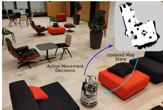
Figure 2.1: Our omnidirectional robot actively maps a reconstructed office reception area.
