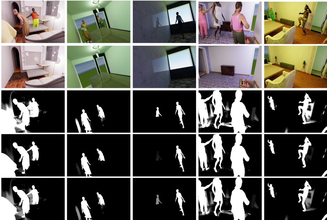
Figure 4.5: Step-by-step visualization of the movable region estimation on multiple synthetic frames, covering shadows, reflections, and movable objects. On the first two rows, we can see the dynamic and background frames. In the third row, we show the result of the clipping operation, while in the fourth row, we report the result of the min-max operation. Finally, on the fifth row, we show the overall result.
