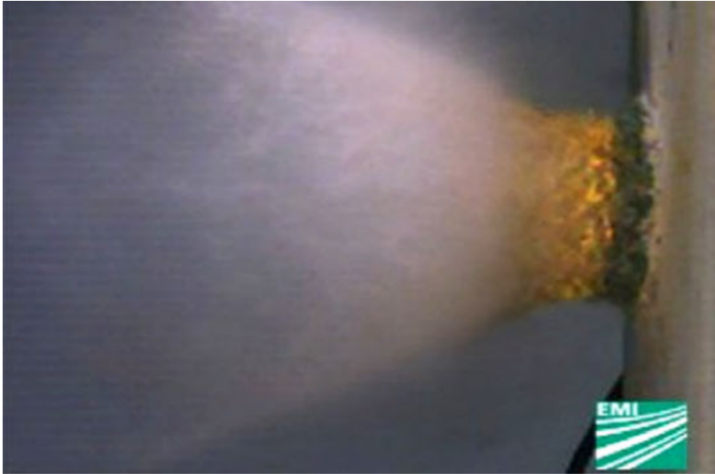
Figure 1.7.: Laboratory experiment of a collision [62, 61] using a two-stage light-gas gun facility. The impact leads to the formation of a crater of about d \approx 10 cm in diameter. The image depicts the ejecta cloud shortly after the impact.
