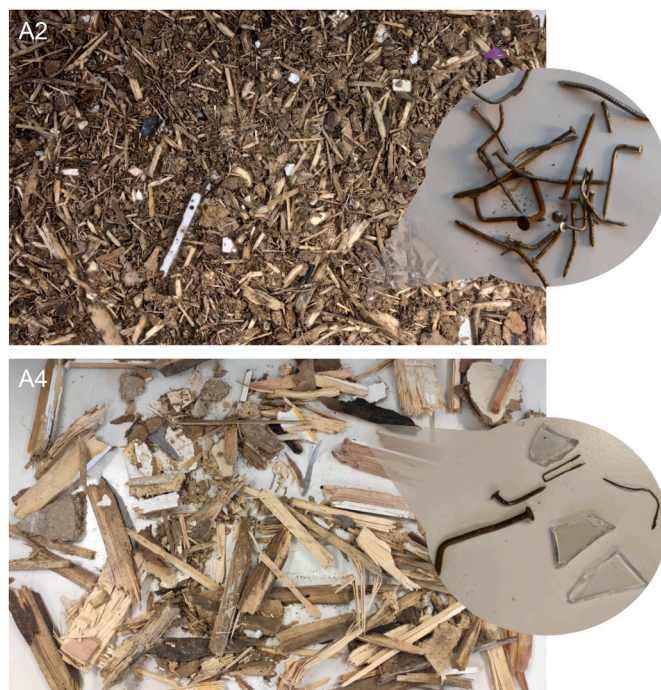
Fig. 1. Examples of the used samples for A1-2a (top) and A4 (bottom) with different impurities.
