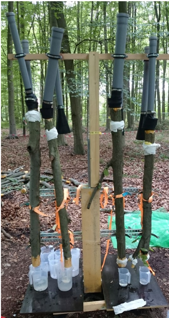
Figure 2 own picture: xylem sap displacement equipment/systematic
