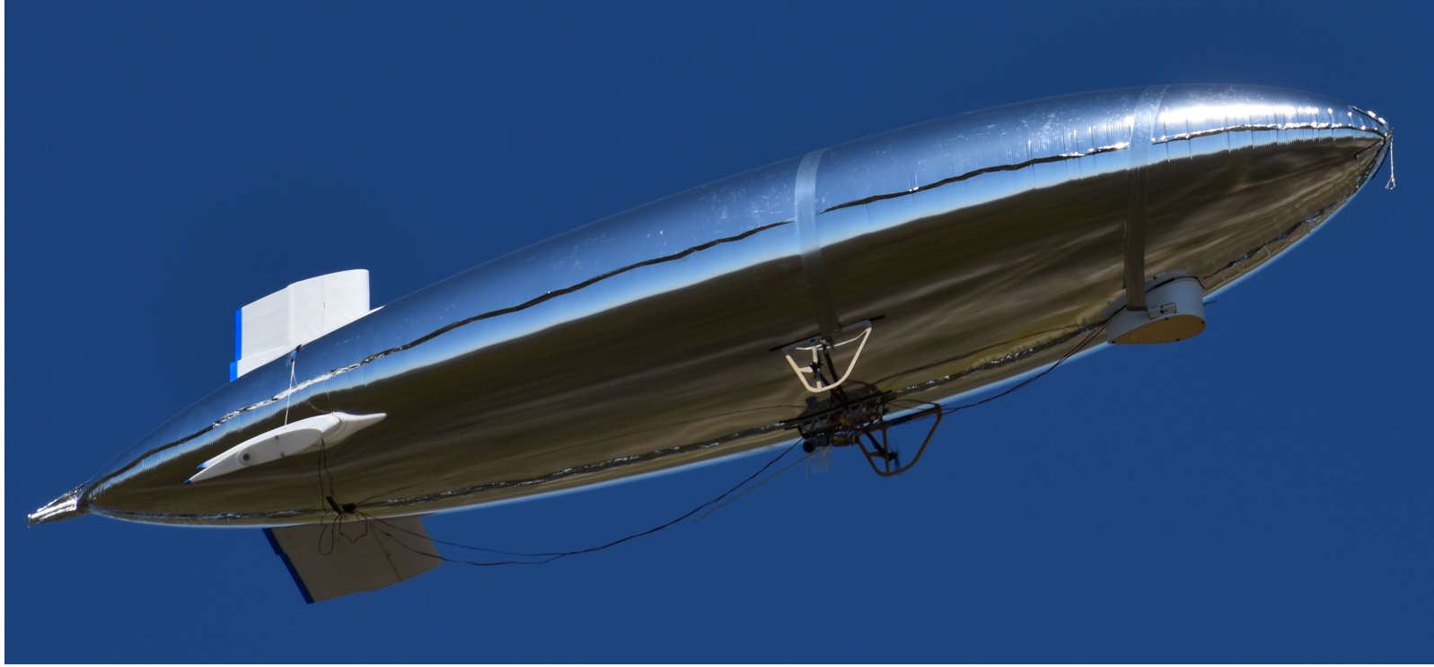
Figure 6.2: Our blimp prototype in the air. This picture shows our airship in flight, picture taken during flight experiments in the Hortobágy National Park, 2023. Clearly visible is the rope attachment we added to the nose as a field modification, as well as the payload and propulsion gondolas, the latter with attached ballast.
