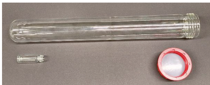
Figure S9. Reaction vessel, based on a 4 ml screw neck vial (Chroma Globe, Kreuzau, Germany) and Schlenk-type tube.
