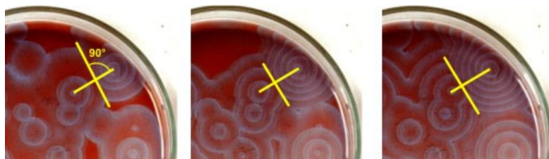
Figure 2.10: Belousov-Zhabotinsky-reaction as a changing wave pattern in a Petri dish. First the solution is red (ferroin indicator \text{Fe}^{2+} ). By a disturbance at one place bromine ions are used up, bromate oxidizes \text{Fe}^{2+} to \text{Fe}^{3+} (ferroin indicator turns blue). Bromine ions diffuse into the surrounding and in this way the red area turns into blue. If the bromine malonate has reduced \text{Fe}^{3+} (bromine ions are formed), the area turns red again. The pictures show at a late situation the pattern changes at 0, 80, and 160 seconds). Released into the public domain by its author, J. Krieger at German Wikipedia Zhabotinsky wave pattern
