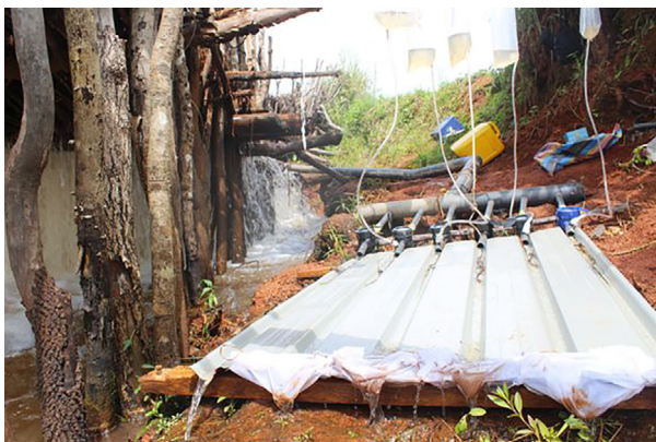
FIGURE 6 Set up of the “System de gouttières” at the local fish trap at the outlet of the lake Bini near the University of Ngaoundéré with plastic bags containing diluted insecticide.
